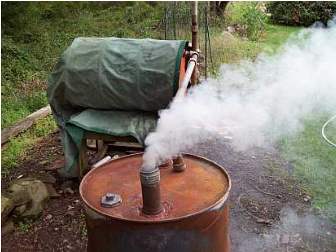
The plugs are removed from the top of the drum to vent the exhaust gases from the burning paper and kindling.
