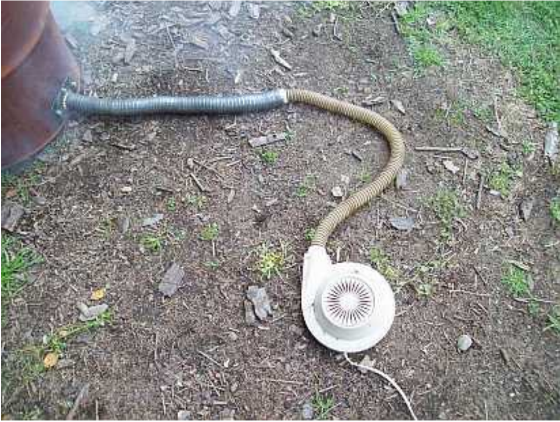
A small blower (old style hair dryer) is attached to the air intake to place a small positive pressure to the drum. This is connected by a piece of flexible steel corrugated tubing.
