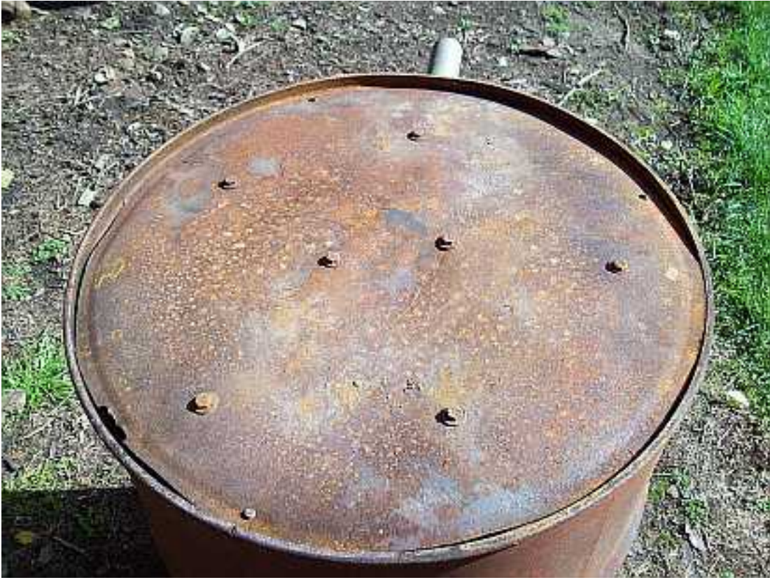
The cover and burning plate is then installed and fastened with a few sheet metal screws..
