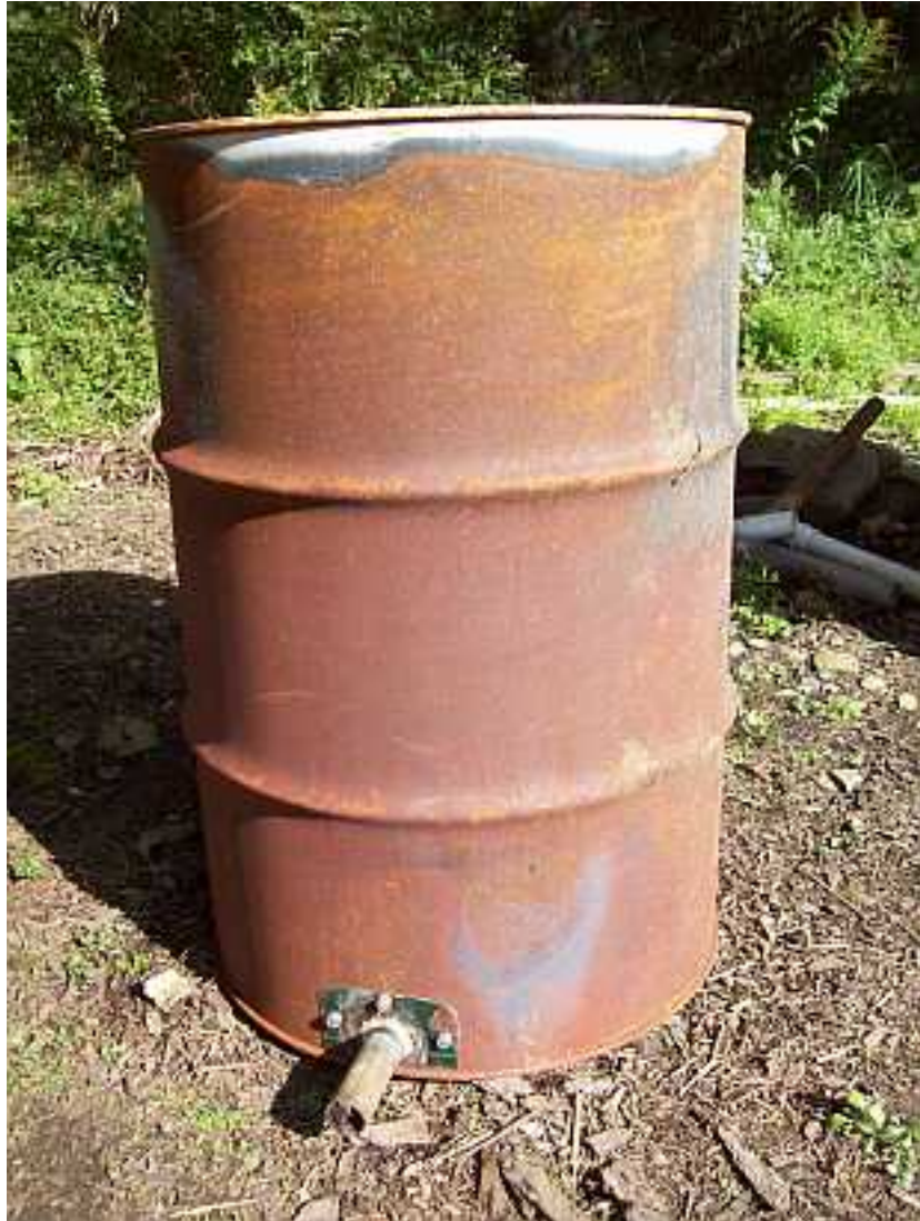
The drum is inverted. The air intake is near the crumpled paper which is now on the bottom.
