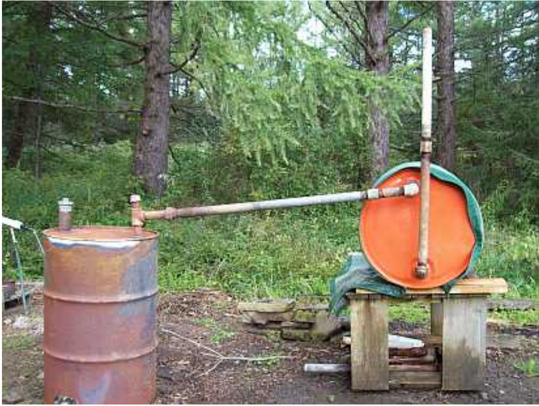
Another 55 gallon drum is used as a condenser and is connected with the appropriate plumbing. The condenser drum is wrapped with wet canvas for cooling.
