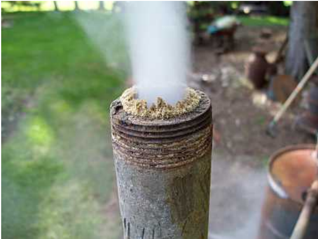
Off-white feathery sublimate clogging the exhaust. This can be found in the entire length of the exhaust plumbing. A sample was saved for analysis.
